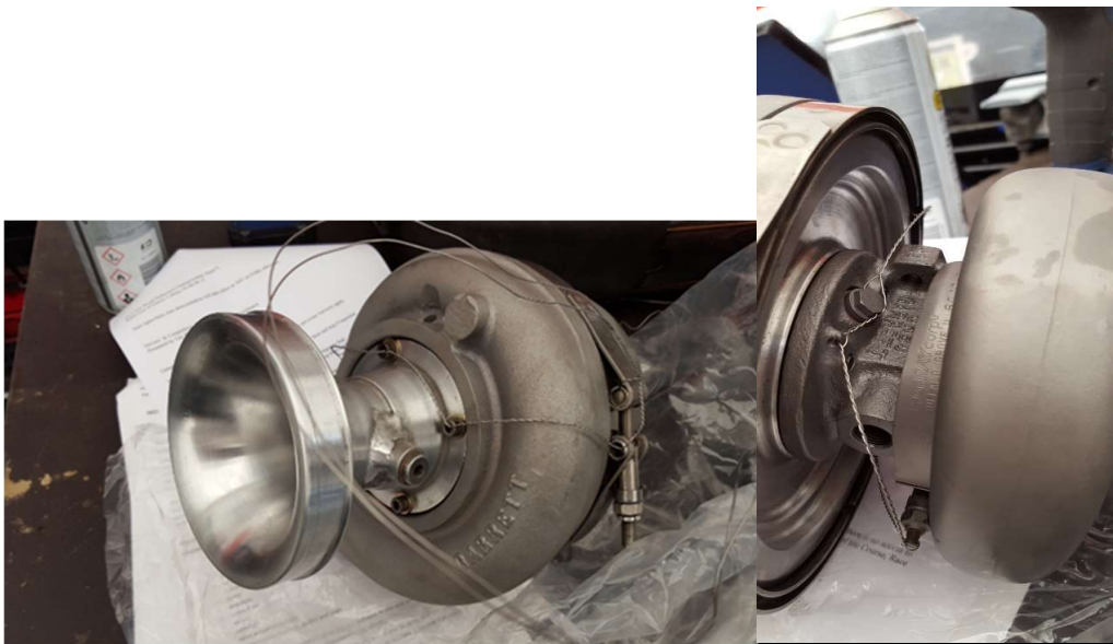
Examples of incorrect sealing wiring
